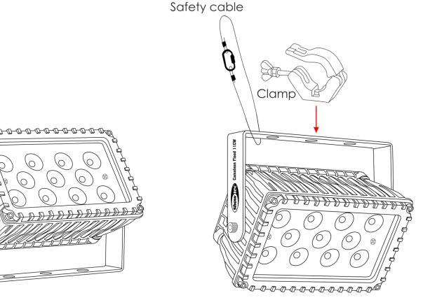
The Cameleon Flood 11CW can be placed on a flat stage floor or mounted to any kind of truss with a clamp.
