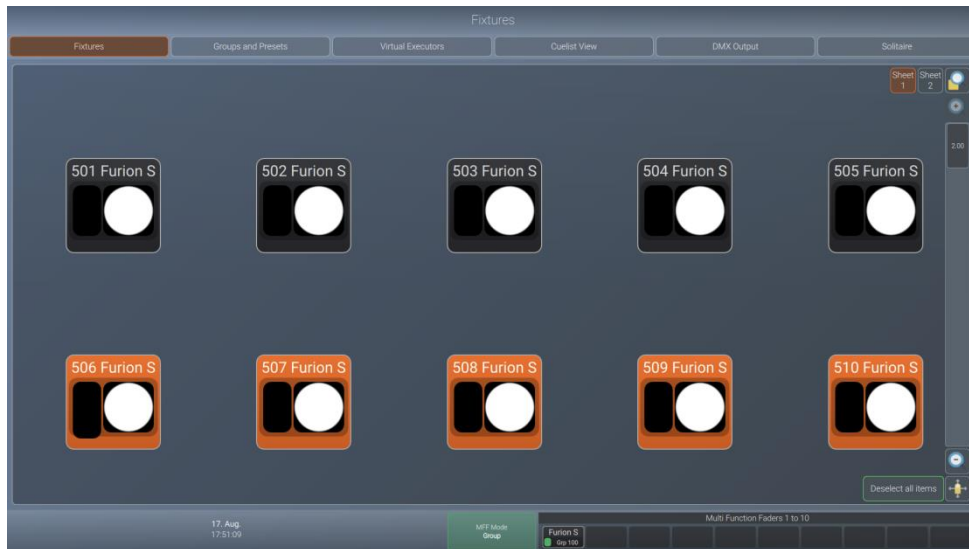
Fig. 21: External Monitor Fixtures View – LAMPY DNGL attached
